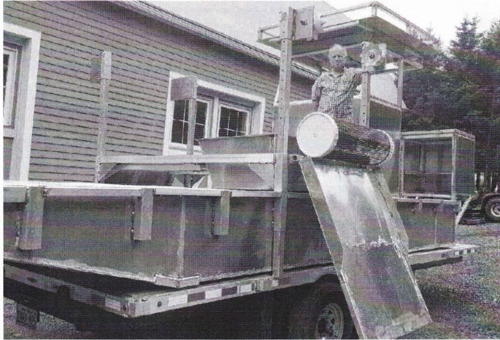
Ernie Porter with the oyster harvester he built in his shop for a proposed aquaculture operation on Antigonish Harbour.
