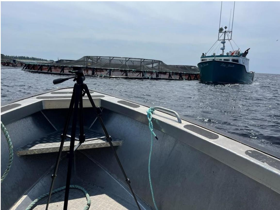
Photograph showing the sound meter set up on the bow of the boat tied up to one of the salmon cages. Other salmon cages and a support vessel at the marine grow-out site can be seen in the background.
