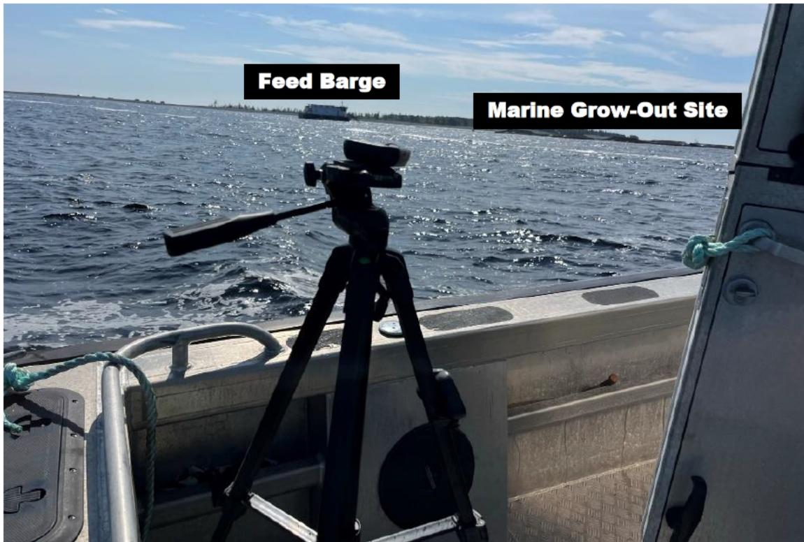
Photograph showing the sound meter set up on the stern of the boat tied up to the northwest corner buoy. The aquaculture marine grow-out site and the feed barge can be seen in the background.
