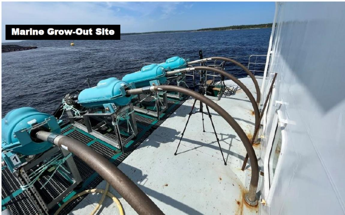
Photograph showing the sound meter set up on the bow of the feed barge near the feed blowers. The aquaculture marine grow-out site can be seen in the background.
