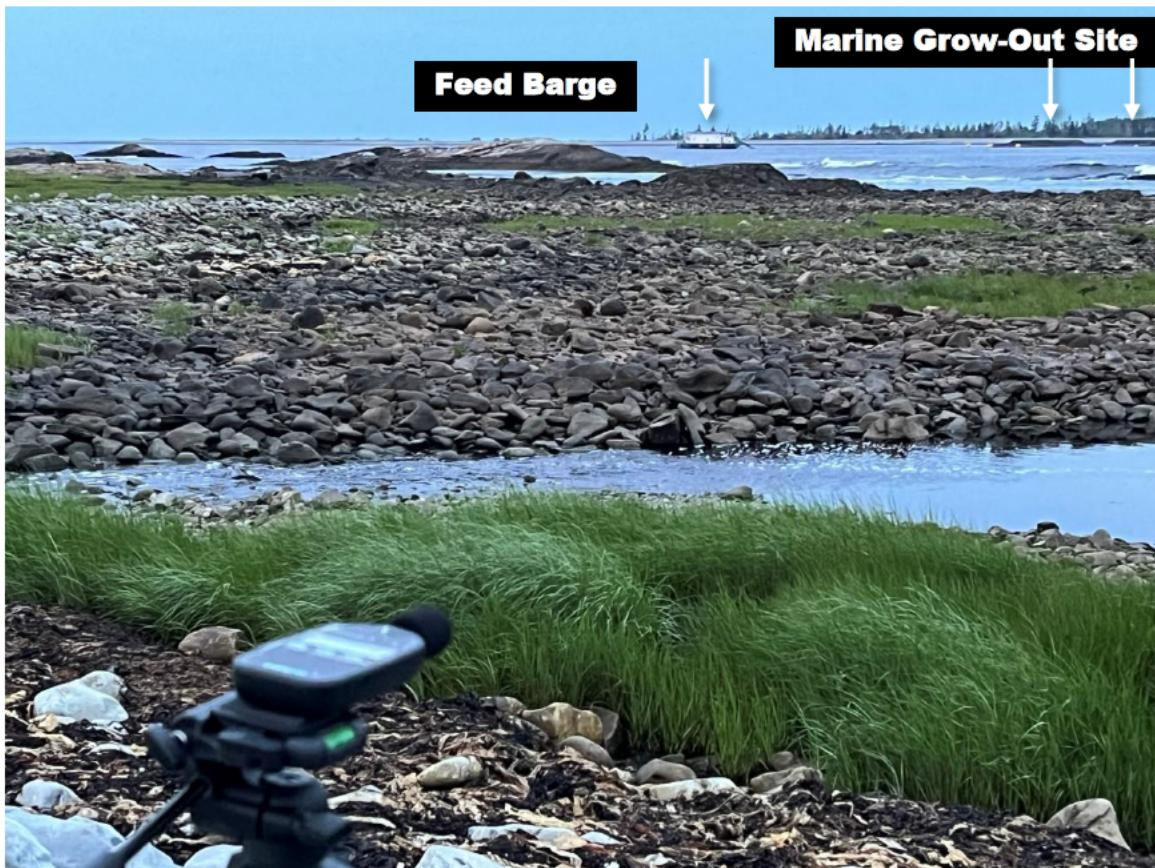
Photograph showing the sound meter set up at the Horse Head Rock sampling location. The aquaculture marine grow-out site and the feed barge can be seen in the background.
