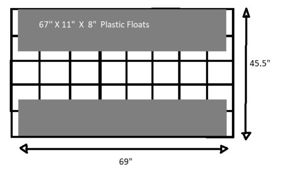
a. Single Structure Schematic – Top View
